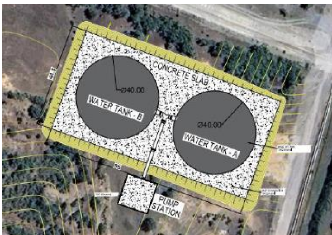
Figure 2.5 Schematic diagram of the preferred low-pressure option of two concrete water tanks.
